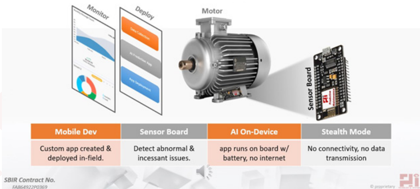
Picture 1: An example of a deployed solution for predictive monitoring and failure detection of critical mud pumps in the oil and gas industry. (Images courtesy of Predictrionics)
